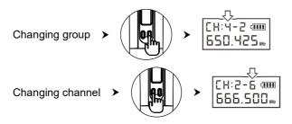
**4** 3 seconds after selecting a channel, it will be automatically saved.
