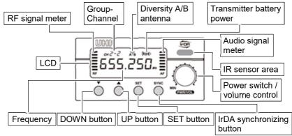
First turn on the power and the LCD display will show last stored group-channel and frequency. Select a channel that corresponds to the transmitter. When transmitter is turned on, the A/B diversity antenna will appear to denote that it is connected.
